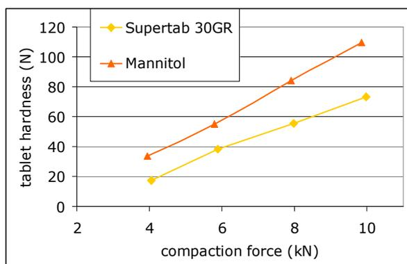
**Figure 3.** Relation of tablet hardness vs. compaction force
