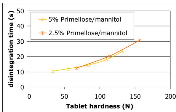
**Figure 4.** Tablet disintegration time of mannitol based tablets with 5% and 2.5% primellose
