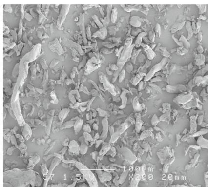
**Figure 2.** SEM picture of Primellose
