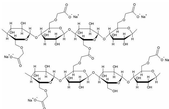
**Figure 1.** Chemical structure of Primellose
