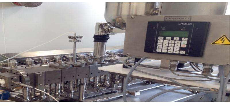
Fig 1: Manufacturing of granules using Leistritz ZSE 18 HPe-VA
