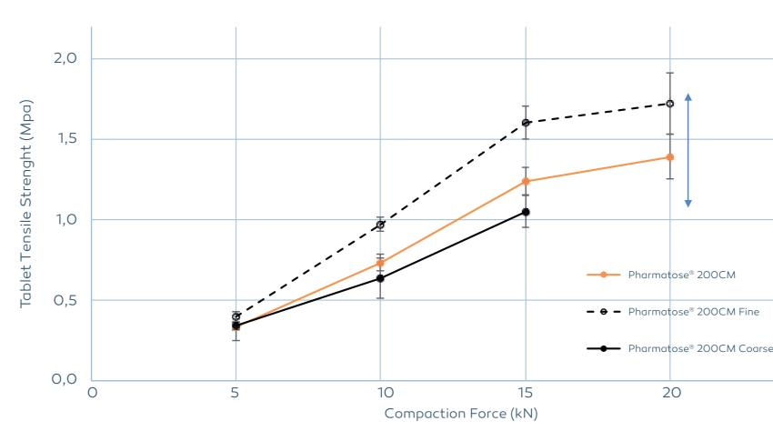
Fig 4: Tablet tensile strength vs Compaction force data of lubricated granules
